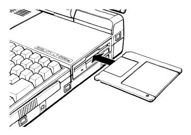
Insert the diskette in the drive so that it clicks into place. When the diskette is all the way in, the release button pops out. For more information on inserting, removing, and caring for diskettes, see Chapter 2. 2. Now press Y and Enter in response to the SETUP program prompt:
